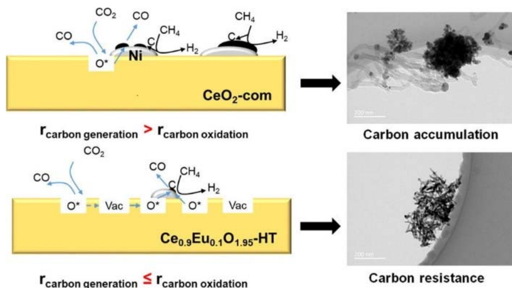
Figure 4. Catalytic mechanism for the reforming of methane by carbon dioxide and the percentage of CH 4 -to-CO and CH 4 -to-coke derived from CH 4 pulse experiments over Ni/CeO 2 -com and Ni/Ce 0.9 Eu 0.1 O 1.95 -HT [81]. O* is a reactive oxygen derived from CO 2 . Copyright 2022, with permission from Elsevier.
