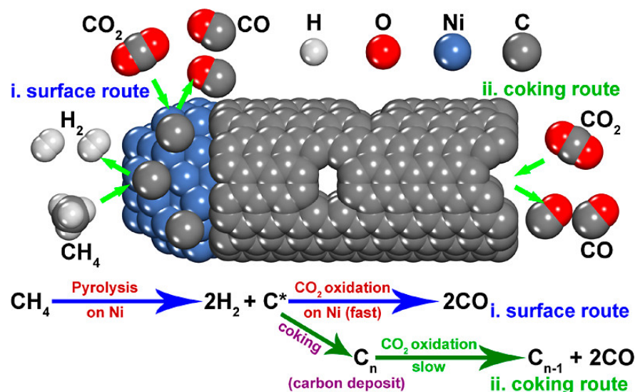
Figure 3. Schematic of the DRM reaction mechanism showing two different routes. The first route (i) is the typically envisioned surface catalytic reaction, whereas the second route (ii) involves the formation and oxidation of coke to produce CO [48]. Copyright 2022, with permission from the American Chemical Society.
