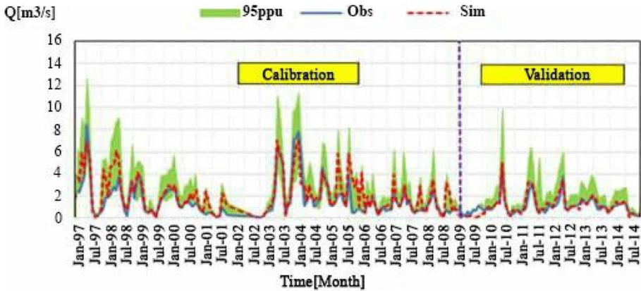
**Fig. 9** Comparison of observed and simulated runoff on a monthly scale in the calibration and validation periods
