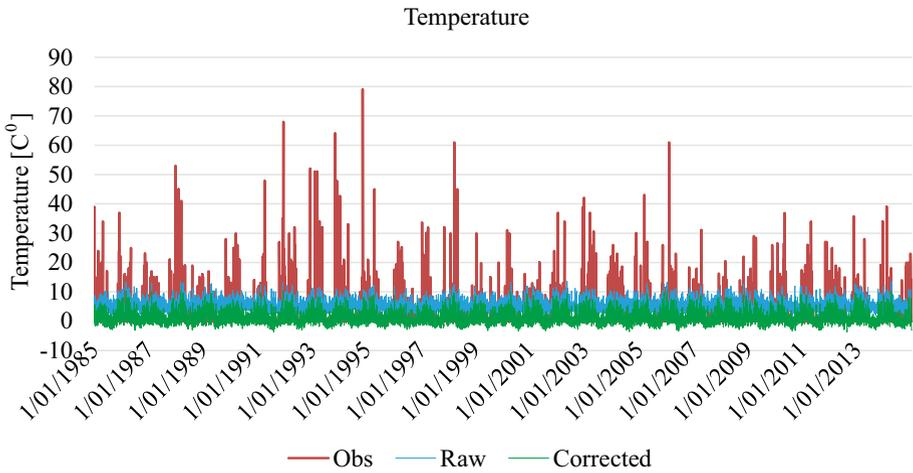
**Fig. 4** Observed, raw and modified values of temperature by LSBC method for Saghez synoptic station in the base period (1985–2014)
