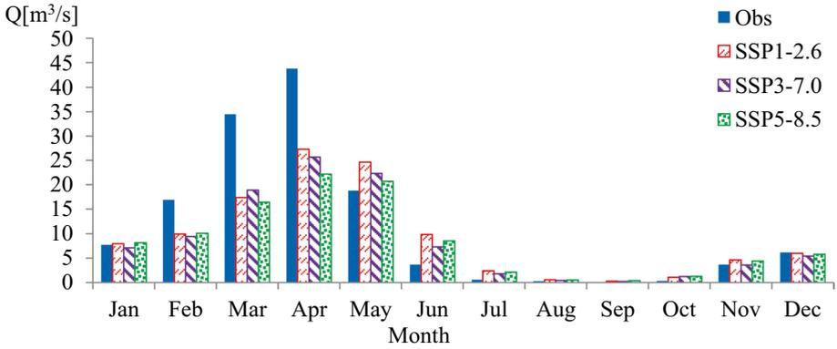
Fig. 13 The surface runoff changes on a monthly basis based on different scenarios in the future period (2021–2050) compared to the base period
