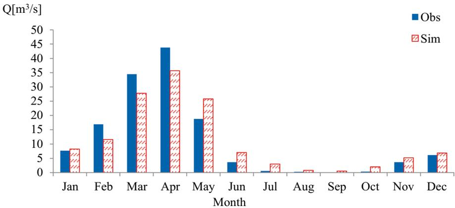
**Fig. 11** Monthly observed and simulated runoff in the base period (1997–2014)
