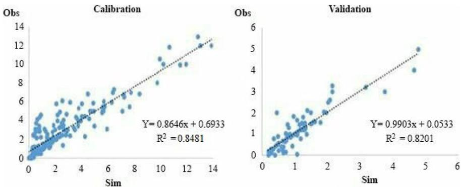
**Fig. 10** Distribution and correlation of observed and simulated discharge values of the model in the calibration and validation periods
