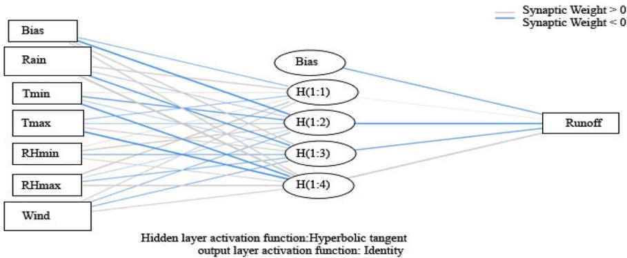
Fig. 6 The structure of the artificial neural network with the best performance in this research
