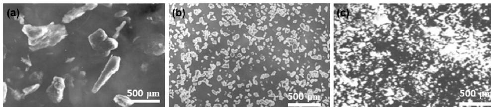
**Fig. 3.** SEM images of (a) bottom, (b) middle, and (c) top region of the casting solidified in the crucible after 10 minutes of holding at 800 °C, for the composite scrap reinforced with 10 wt% SiC particulates of size 125 μm.
