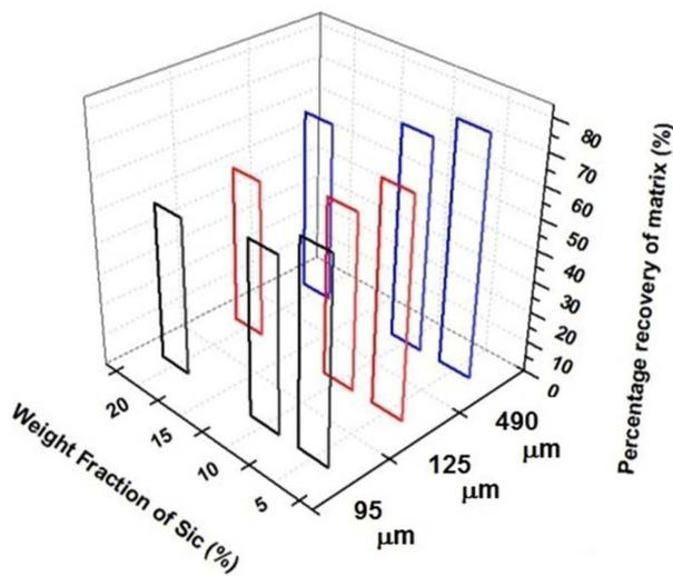
**Fig. 5.** Influence of SiC particulate size and amount on maximum percentage recovery of Al alloy.
