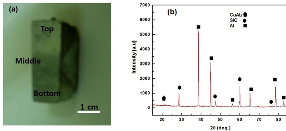
**Fig. 2.** (a) Image take from the bottom of solidified casting in the crucible after 10 minutes of holding at 800 °C, for the composite scrap reinforced with 5 wt% SiC particulates of size 125 μm, (b) XRD pattern of (a) in the middle region.
