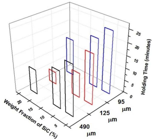
**Fig. 6.** Influence of SiC particulate size and amount on minimum holding time required to achieve maximum recovery of Al alloy.
