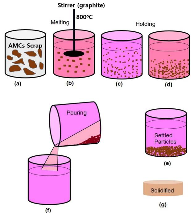
Fig. 1. Schematic diagram for separation of Al matrix and SiC reinforcement.
