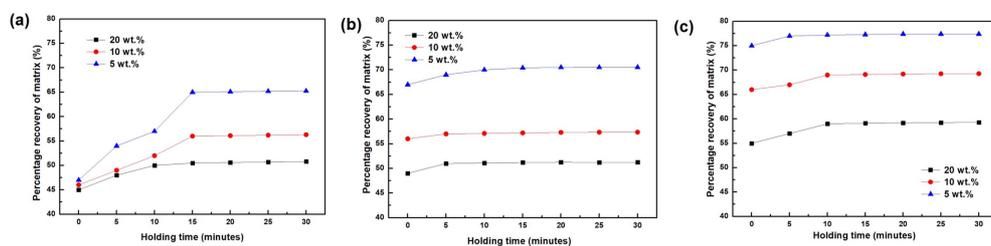
**Fig. 4.** Relationship between the SiC weight fraction and recovered Al matrix for SiC particulate size, (a) 95, (b) 125, and (c) 490 μm.
