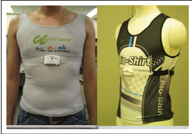
Figure 5. Fall detection method using a fixed accelerometer sensors. 14
